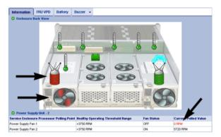
In this example, a power supply fan has stopped turning, indicating a failure. The Enclosure Diagram displays color and motion changes to identify a failed fan. In this case, you must replace the power supply.
